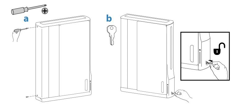
a. Slide door to the left and remove these 3 screws. Save screws for reattaching cover. b. Remove left cover.
