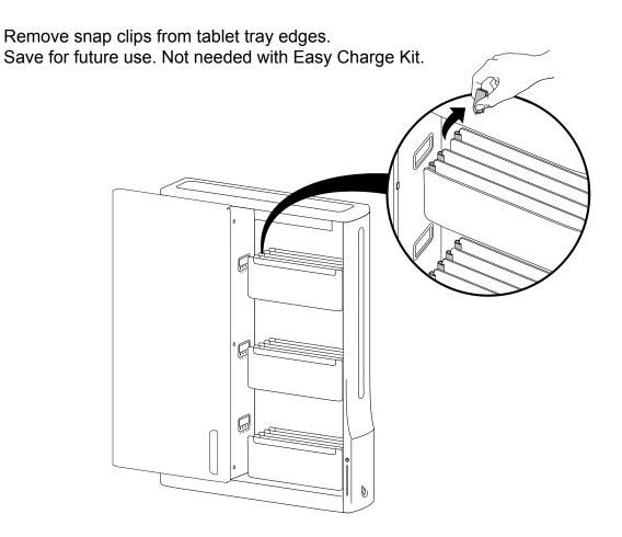
Place Easy Charge tray into tablet tray with the curved side towards the outer wall and cables on the left side. Press into place and listen for snaps to engage. Feed cables through holes in side wall.
