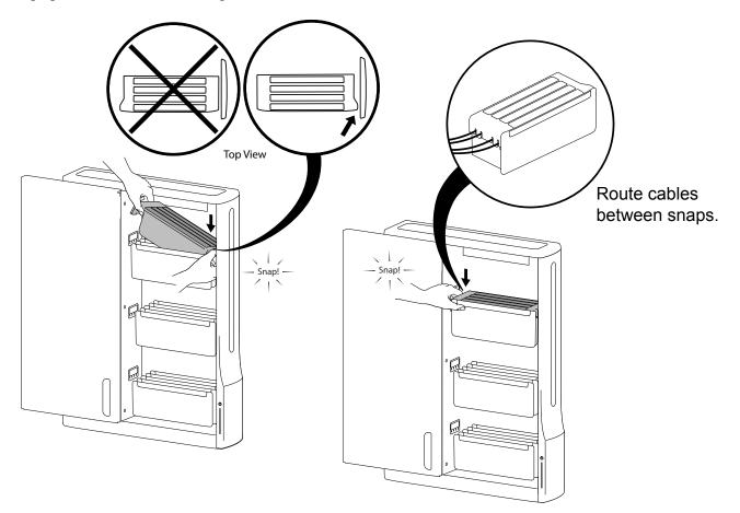
5 Pull USB cables through outer wall. Make sure cables are positioned one per slot and attach to USB wall chargers.
